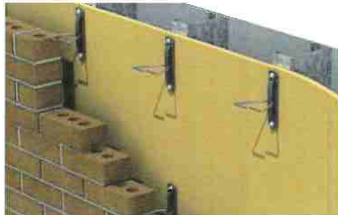
Diagram showing how masonry ties are to be anchored.
